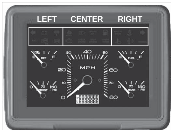
Figure 8 Indicator Lights on the Main Gauge Panel
