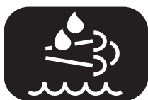
Figure 27 Diesel Exhaust Fluid (DEF) Lamp
