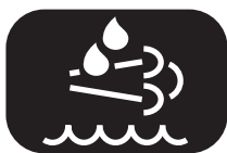
Figure 28 Diesel Exhaust Fluid (DEF) Lamp
